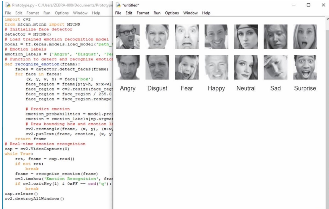
Figure 4.2: Emotion Results (a) seven emotions detected by the system using the CK and FER2013 datasets
